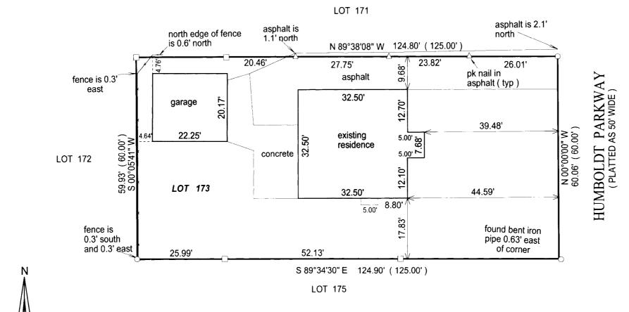
( )= recorded as  $\Box$  = found iron bar = found iron pipe = set iron pipe = set iron bar SCALE 1" = 20' 20
